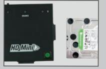
2.Plug in the source HDD and target HDD(s). The correspondentLED will be on if the HDD is connected well.
