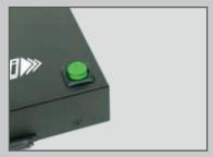
**3.**Press down the green button, the HD Mini will start duplication automatically and the LED(s) will keep flashing.
