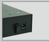
**1.**Plug in the power adapter (the other side of the power adapter should be plugged into a power outlet) and turn on the power switch.
